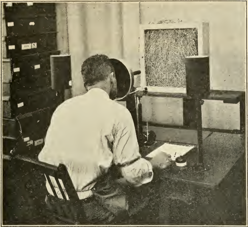
FIGURE 17.—A simplified instrument recently developed for measuring the color of hay. An area of the hay 14 inches in diameter may be measured at one time
